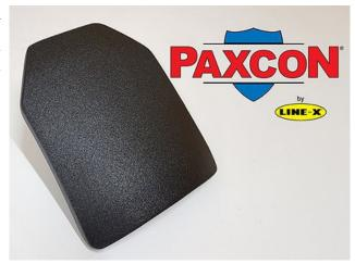
➤ The flexibility and absorption that LINE-X Spall Liner offers when applied to armoured panels eradicates the splintering effect by cushioning the impact and entrapping the fractured elements. PAXCON spall lining is currently being used on armoured vehicles in conjunction with Dyneema and similar armoured panels which is significantly lighter and more cost effective than armouring with steel plates.
