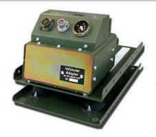
➤ The manpack vehicular adapter BV-5800 provides the ability to connect the manpack to the antenna in vehicular and shipboard applications. The adapter allows a standard RF-5800 series manpack radio to directly connect to the antenna without an external power amplifier. The adapter is designed for applications that require nominal RF (radio frequencies) power.
