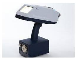
**RoadRunner** is designed to detect traces of explosives and drugs on surfaces of objects and parts of the body, DE-tector flex is able to detect and identify substances that are measured in some nanograms. Is widely used at airports for screening passengers and cargo, customs checkpoints and other strategically important objects.
